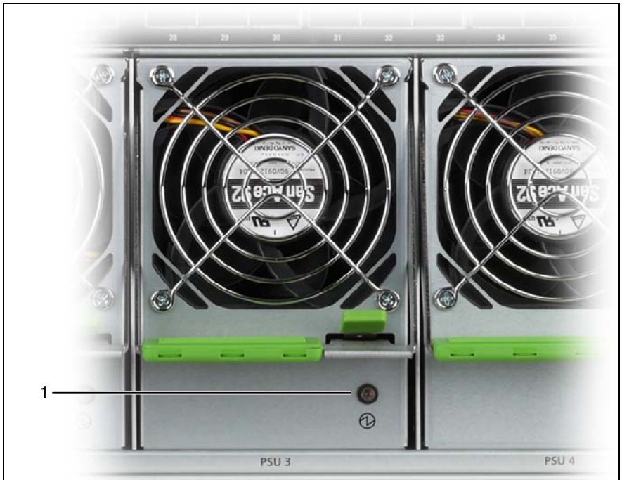
Figure 18: Indicators on the hot-plug fan module
